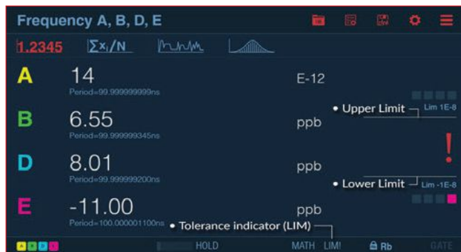
▲ Fig. 2 Four simultaneous signals on CNT-104R display.
